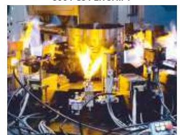
AUTOMATIC FLASK FORMING MACHINE: 800 PCS PER SHIFT
